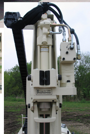
The Geoprobe® GH42 percussion hammer system (Right)
